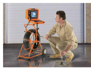
In addition to the card reader, the Gen-Eye SD includes an 8" LCD color monitor for crisp, clear pictures, a full keyboard for on-screen titling, on-screen distance counter, built-in voice over unit, date and time stamp, LED dimmer control, camera test port, and both AC and DC power cords. All are safely contained in a padded case weighing just 10 lbs. that can stand alone or mount on a reel.
